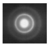
Fig. 2.13: Electron diffraction pattern from nickel crystal
