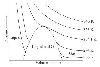
Figure 5.14: Isotherms of carbon dioxide
