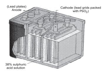
Fig. 13.11: Lead storage battery
