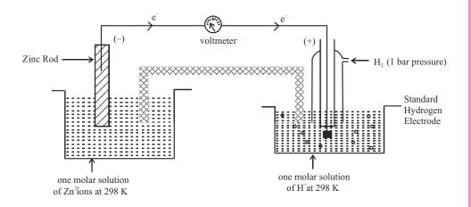
Fig. 13.9: Measurement of standard electrode potential of Zn/Zn<sup>2+</sup> electrode
