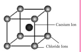
Fig. 6.21: Caesium chloride structure
