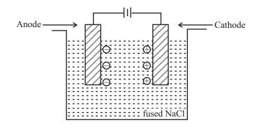
Fig. 13.4: Electrolytic cell
