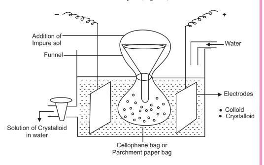
Fig. 8.4: Electrodialysis
