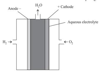
Figure 13.12: Hydrogen-oxygen fuel cell
