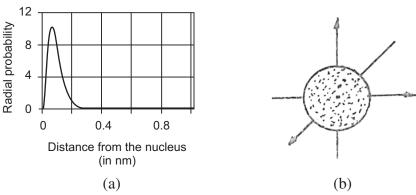
Fig. 2.14: (a) Radial probability curve for 1s orbital (b) Boundary surface diagram for 1s orbital
