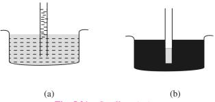
Fig. 5.21: Capillary Action
