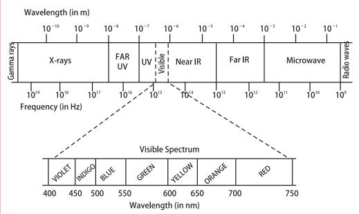
Fig. 2.7: The electromagnetic spectrum
