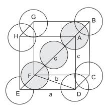
Fig. 6.19. Body centred cubic until cell.
