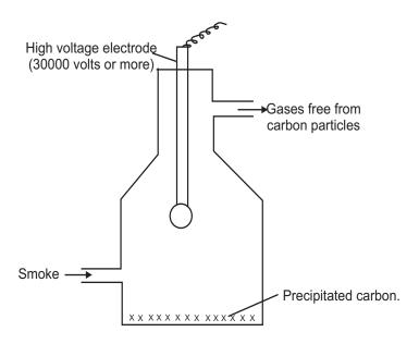
Fig.8.8: Cottrell smoke precipitator
