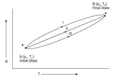
**Fig. 9.2 :** Change of state from initial state to final state through three paths I, II and III. The difference  $p_2 - p_1$  and  $T_2 - T_1$  are independent of the path since pressure and temperature are state functions.
