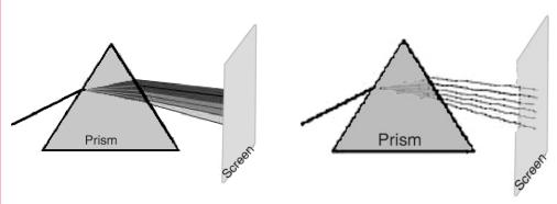
Fig. 2.8: a) a Continuous spectrum
