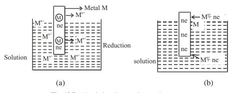
Fig. 13.7: Metal placed in a solution of its ions
