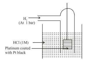
Fig. 13.8: Standard Hydrogen electode
