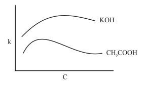
Fig. 13.2: Variation of conductivity with concentration
