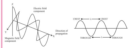
**Fig. 2.6:** (a) An electromagnetic wave showing electric and magnetic fields travelling in planes perpendicular to each other and also to the direction of propagation (b) Characteristics of electromagnetic wave
